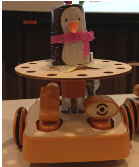
Figure 7: New KIBO robot with updated color and new motorized art platforms for personalizing. It is shown here decorated with arts and crafts to represent a penguin.
