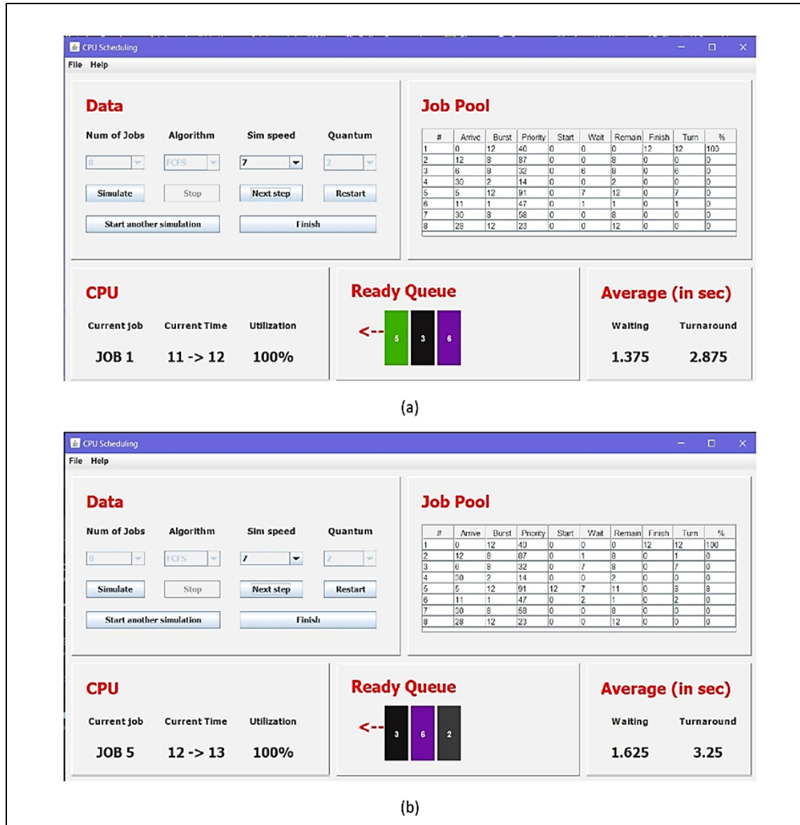
Figure 24. Ready queue for two simultaneous steps
