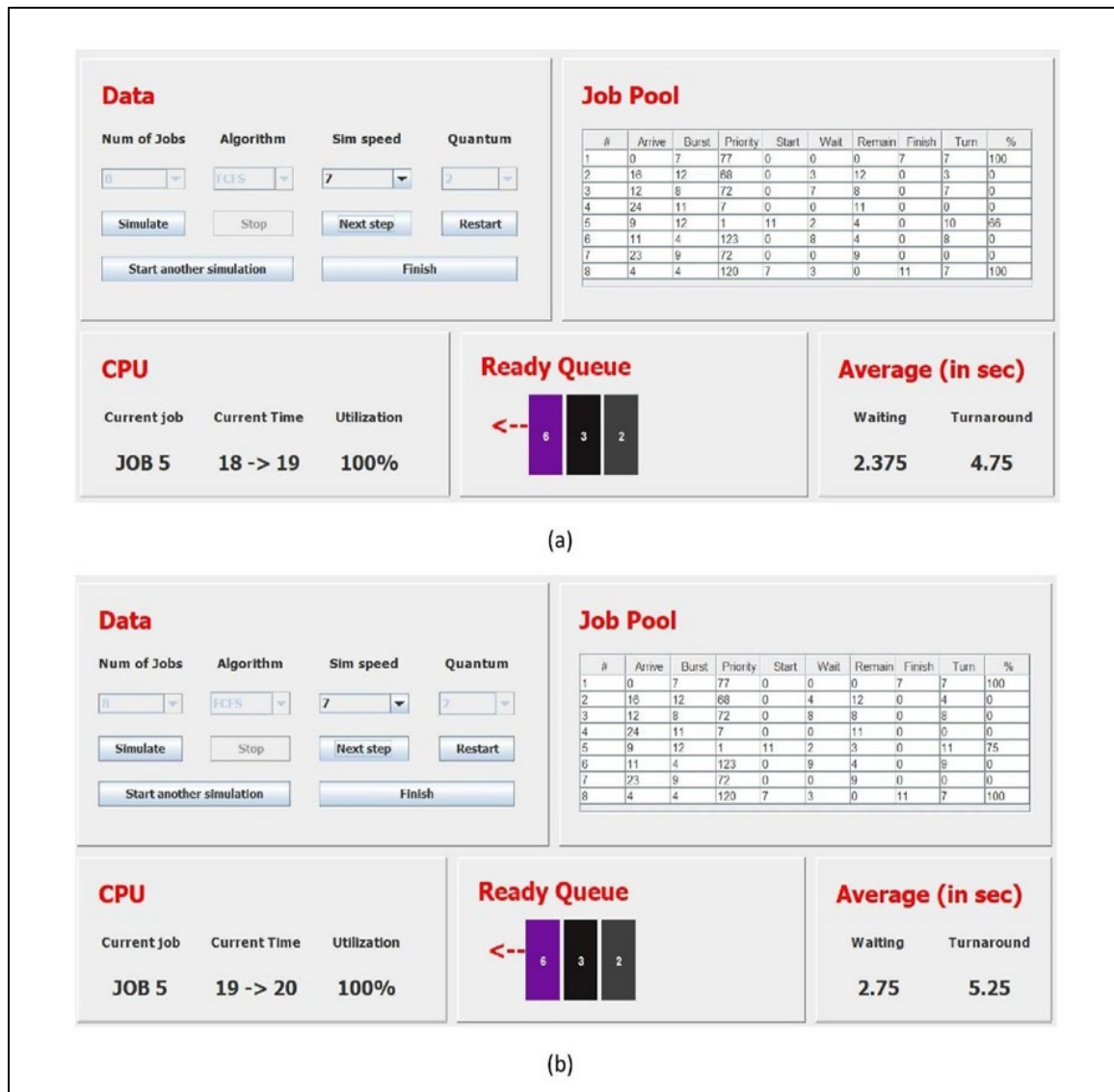
Figure 22. Calculation of waiting time and turnaround time (in seconds) at each step
