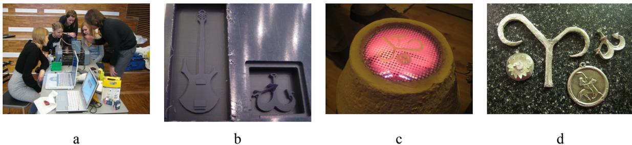
**Figure 6:** *The process of silver jewelry fabrication: a) wax cast producing with Modela milling machine; b) samples of wax casts; c) silver clay objects fired on a portable kiln; d) final silver artefacts.*
