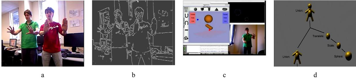
**Figure 5:** *Kinect FRep Modeller concepts: a) user control with hand gestures; b) hands detection using a Kinect camera; c) a cursor attached to either hand; d) constructive modelling using the menu of primitives and operations.*
