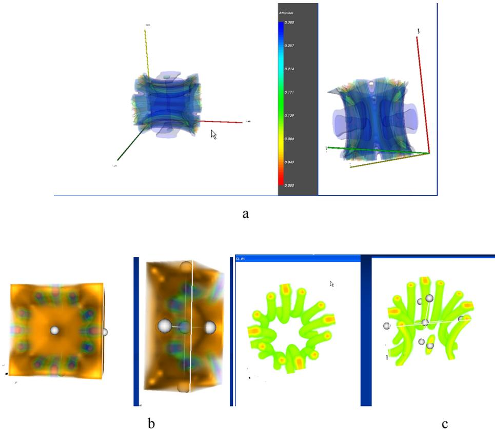
**Figure 8:** Scientific visualization example for the order-parameter field for the second type superconductor (Abrikosov vortices). Different approaches to scalar field visualization: a) isosurfaces; b) volume visualization with the scalar field defined on a rectangular domain; c) scalar field on a complex domain defined by one of the field's isosurfaces. The field's domain can be interactively cross-sectioned by the user with planes controlled by white handles.
